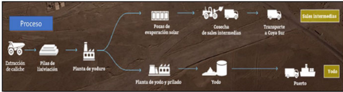
Figure 15-3. Nueva Victoria Plant Process Diagram
