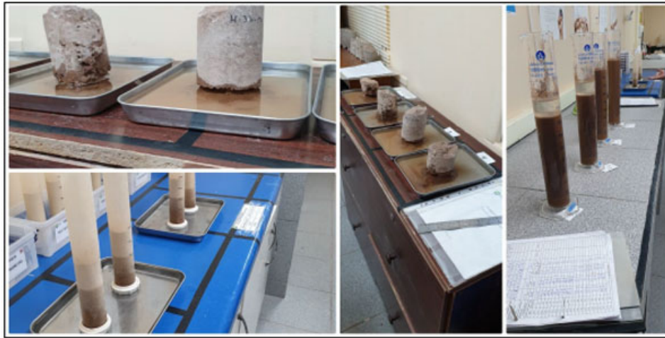
Figure 10-3. Embedding, Compaction, and Sedimentation Tests Performed in the Iris Pilot Plant Laboratory
