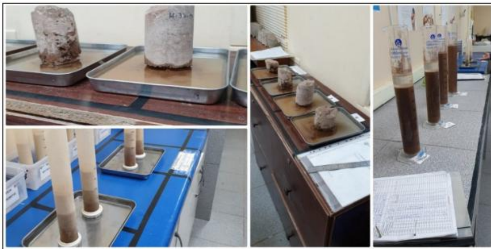
Figure 10-4. Embedding, Compaction, and Sedimentation Tests Performed at the Iris Pilot Plant Laboratory
