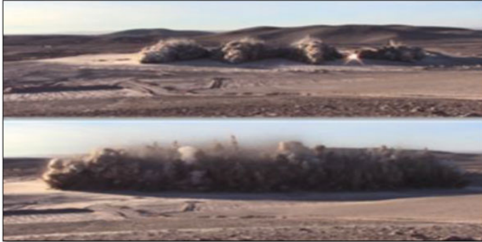
Figure 13-5. Typical Blast in Nueva Victoria Mine (caliches)
