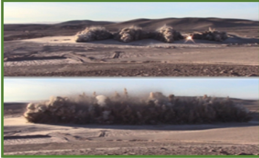
Figure 13-5. Typical Blast in Nueva Victoria Mine (caliches)
