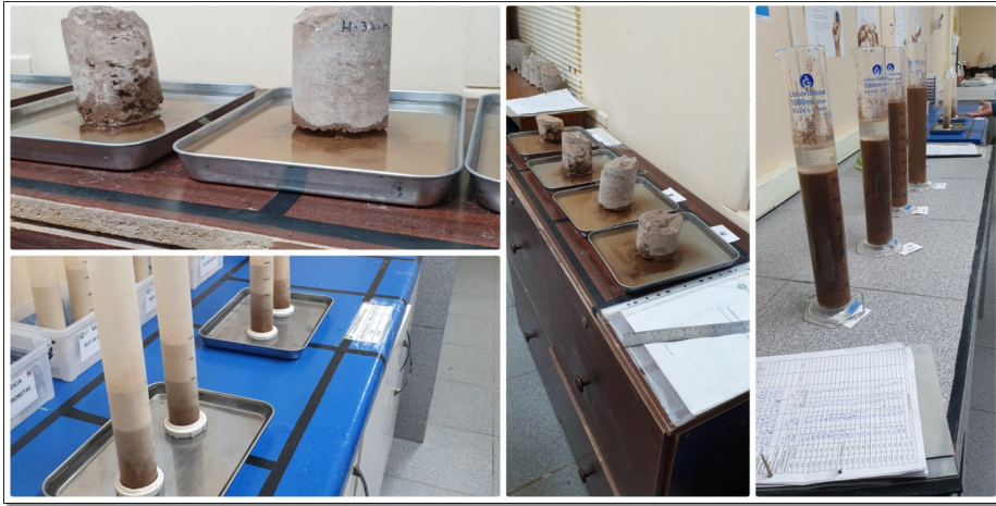
Figure 10-5. Embedding, Compaction and Sedimentation Tests carried out in the Iris Pilot Plant Laboratory.
