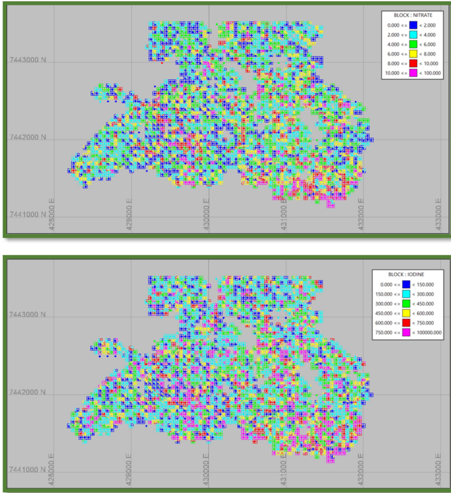
Figure 11-7. Visual Validation of Iodine (Up) and Nitrate (Down) Estimation, Plan View – PB5
