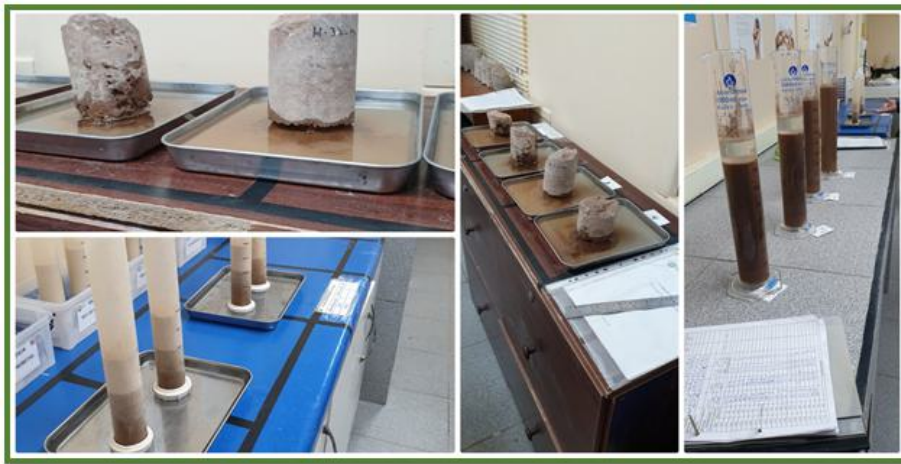
Figure 10-5. Embedding, Compaction and Sedimentation Tests Performed in the Iris Pilot Plant Laboratory.
