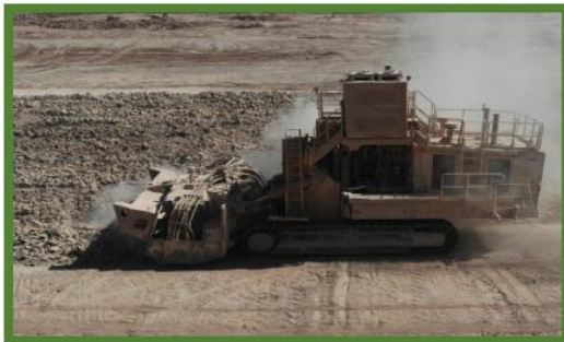
Figure 13-3. Terrain Leveler and SME equipment (Vermeer)
