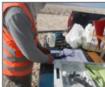
d) pH, temperature, and conductivity measurement
