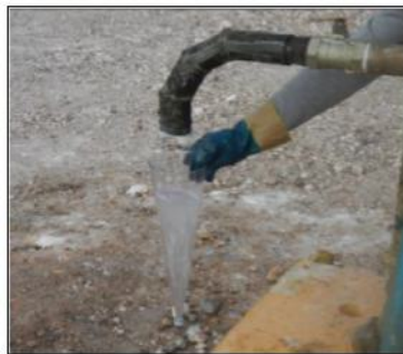
b) Clarity and fine sediment measurement
