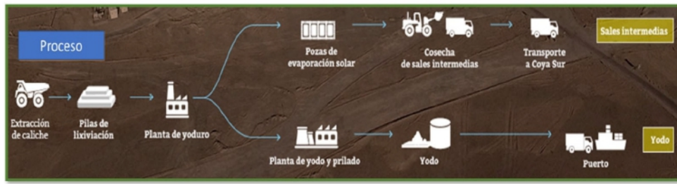
Figure 15-3. Nueva Victoria Plant Process Diagram
