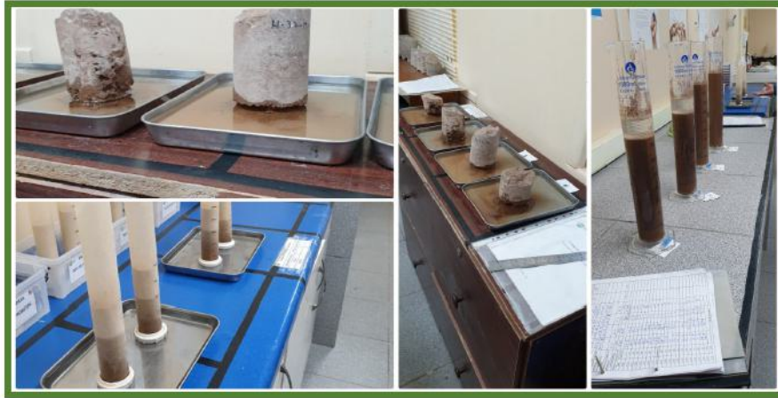
Figure 10-6. Embedding, Compaction and Sedimentation Tests Performed in the Iris Pilot Plant Laboratory.
