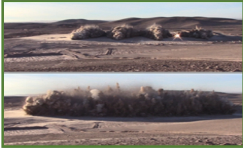
Figure 13-5. Typical Blast in Nueva Victoria Mine (caliches)
