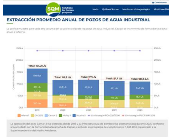
Figure 17-4. Industrial Water Consumption, Total Authorized Limit and Authorized Limit in the Different Wells
